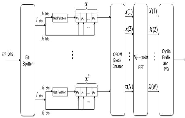
Figure 1. Transmitter structure of OFDM-SPM scheme.
