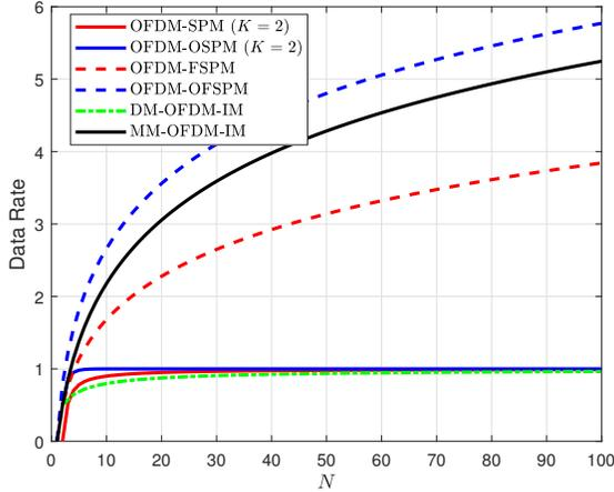
Figure 2. Data rate comparison of OFDM-SPM variants with DM-OFDM-IM and MM-OFDM-IM.
