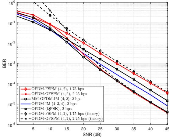
Figure 4. BER comparison of OFDM-FSPM (4,2) and OFDM-OFSPM (4,2) with MM-OFDM-IM (4,2), OFDM-IM (4,3,4) and OFDM (QPSK).
