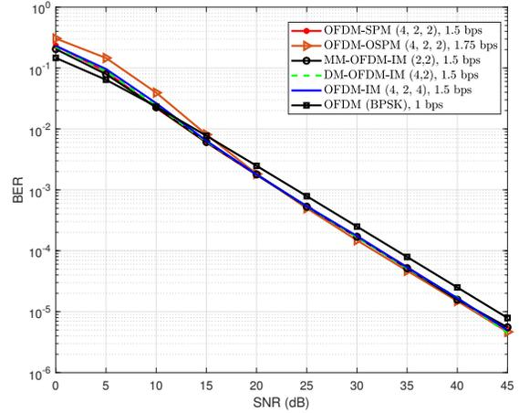
Figure 3. BER comparison of OFDM-SPM ( $4, 2, 2$ ) and OFDM-OSPM ( $4, 2, 2$ ) with MM-OFDM-IM ( $2, 2$ ), DM-OFDM-IM ( $4, 2$ ), OFDM-IM ( $4, 2, 4$ ) and OFDM (BPSK).
